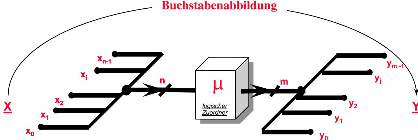
$$y_0 = f(x_0, x_1, \dots, x_i, \dots, x_{n-1})$$
