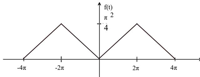
$$\begin{aligned} c_0 &= \frac{2}{T} \int_0^{2\pi} f(t) dt \\ &= \frac{2}{4\pi} \int_0^{2\pi} \frac{\pi}{8} t dt \\ &= \frac{1}{16} \frac{1}{2} [t^2]_0^{2\pi} \\ &= \frac{1}{32} 4\pi^2 = \frac{1}{8} \pi^2 \end{aligned}$$
