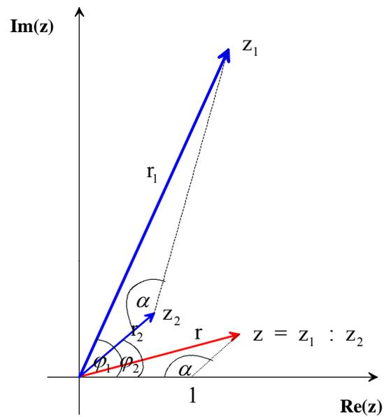
$$r : 1 = r_1 : r_2 \Rightarrow r = r_1 : r_2 \quad \text{und} \quad \varphi = \varphi_1 - \varphi_2$$
